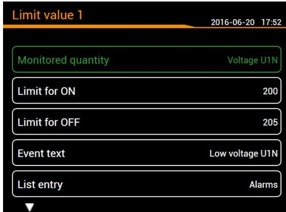
Using limit values either the exceeding of a given value (upper limit) or the fall below a given value (lower limit) is monitored.
