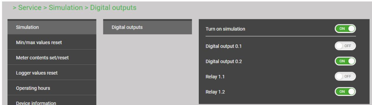
Simulation of digital outputs via device webpage
