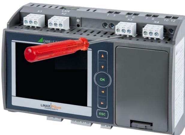
You may have to remove first the plug-in terminals to get access to the screw terminals of the current inputs.
