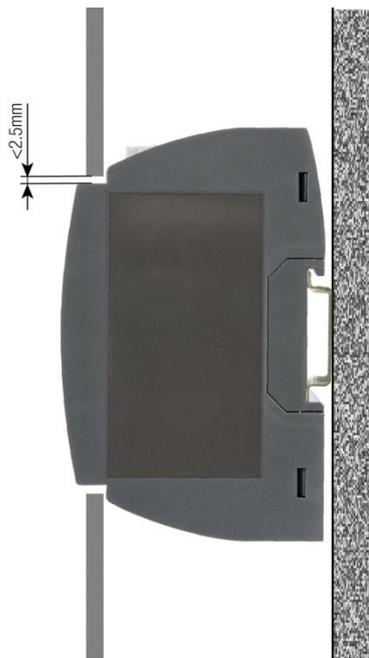
The device can also be mounted that the front of the device protrudes through a cut-out in the enclosure. So the operating buttons and the display become accessible. With centric mounting using the below maximum cut-out a gap between enclosure and device results, which does not exceed 2.5mm on each side.
