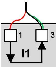
In order to suppress injected interferences, the shielding (green) is connected always to the I terminal of the current inputs (terminals 3, 6, 9, 12).
