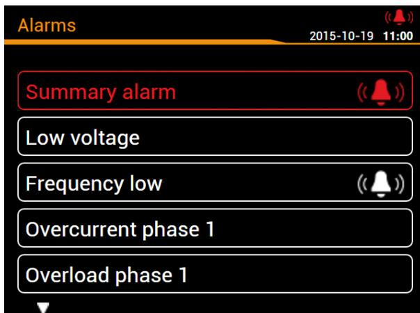
The digital or relay output assigned to the summary alarm can be reset by means of the <OK> key. So the active alarming will be stopped. But the alarm state of the summary alarm remains active until the alarm state no longer exists.
