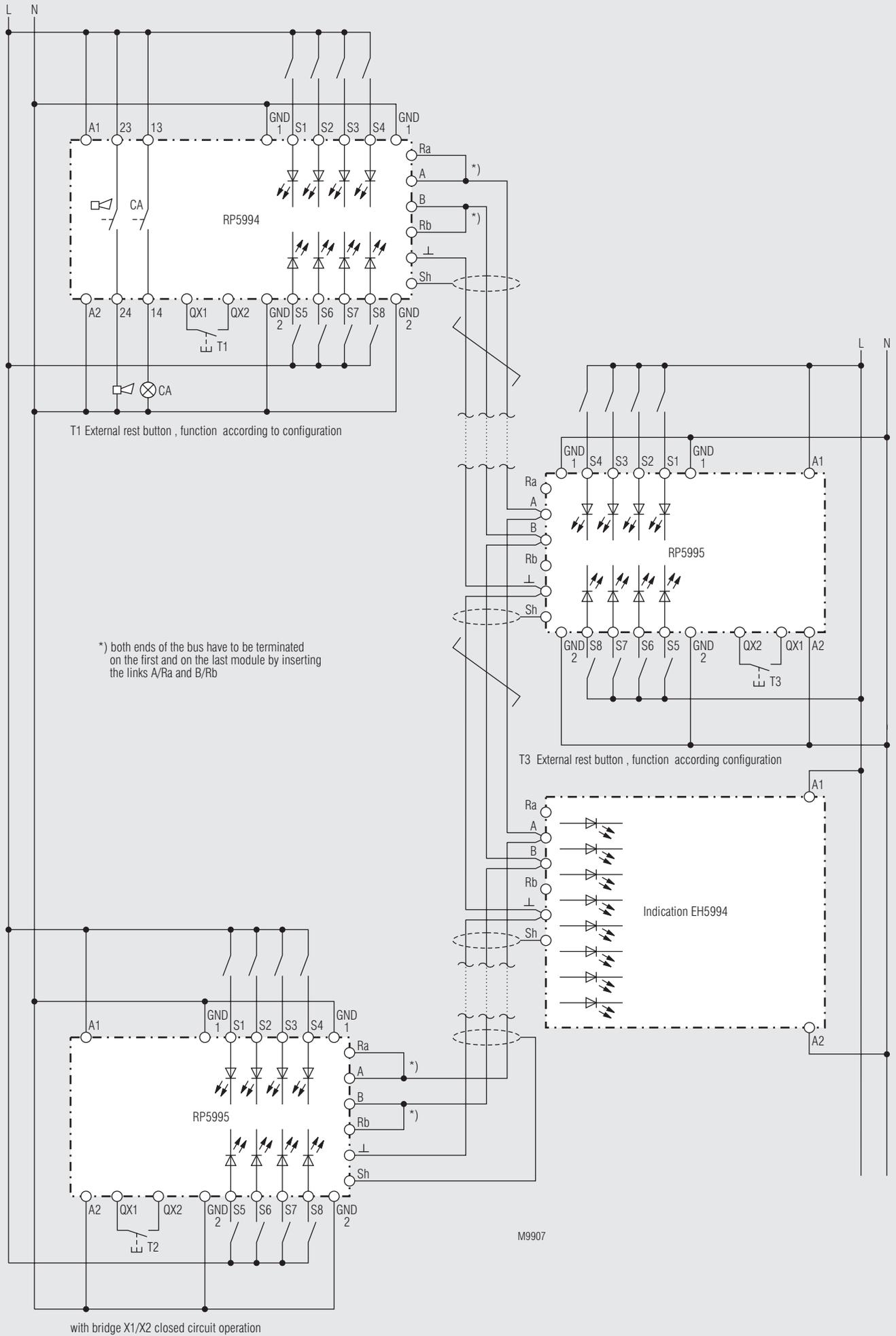
\*) both ends of the bus have to be terminated on the first and on the last module by inserting the links A/Ra and B/Rb
