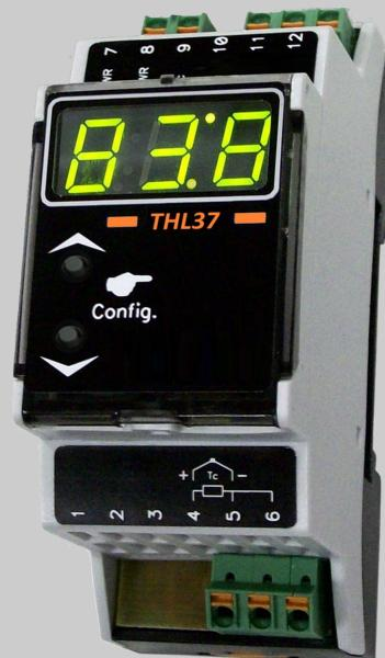
The THL36 is a compact digital thermostat, designed for simple temperature regulation of heating elements (cable, ribbon), allowing the direct control of resistive load up to 4.5 KWatt. The numeric regulation combine accuracy and ease of use. The temperature and the setpoint are displayed on large LED display
